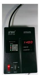
This model is designed for Indication of water level of tanks as well as other related parameters i.e. Flow status, Overflow alarm, Full Level alarm, Low Level alarm for single/ multiple tanks (Maximum 5 Tanks) with audio buzzer for alarm. This is suitable for Housing Societies/ Hospitals/ Institutions/ Schools/ Colleges & Factories with multiple tanks. [Size in mm: 220(H) x130(W)x42(D)]
