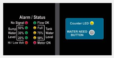
No Signal: This LED will blink if it dose not receive signal from sump tank transmitter and glow steadily, if it dose not receive signal from O.H Tank transmitter. If it is receiving signal from both transmitter it will remain off.
