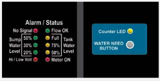
This model is designed for controlling the motor which pump water from sump tank to over head tank.
