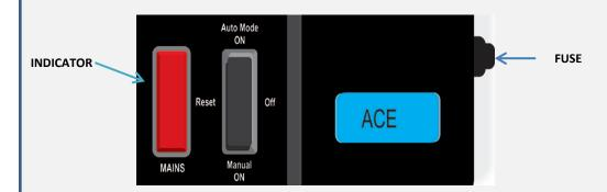
Main Switch: This is three stop switch. When pressed at top most position the controller will operate in Automatic Mode. When this switch is pressed at lower most position it will be in manual mode and the motor will be started. At center position of switch, the controller will be Off. To reset the controller the switch should be in off position for 5 sec. and afterward in "Auto-Mode" position.
