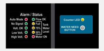
Auto Mode: If it is glowing, it indicates that controller is working in automatic Mode i.e it will perform all operation automatically.
