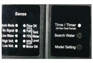
Search Water (Button No-1): Press this button for 5 seconds to trigger the motor and check water supply. Mode/ Setting: Its for internal settings.
